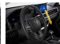
Tilt control of steering wheel angle
